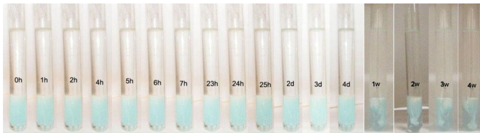
Figure 83 - Evolution of the emulsion using 2% of N6N3 particles from 0 hours to 4 weeks
