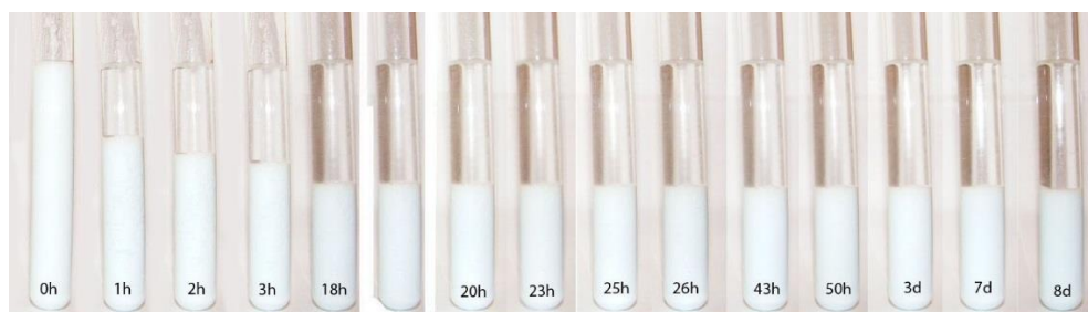
Figure 51 - Evolution of the emulsion using 4g of Pluronic P123 from 0 hours to 8 days
