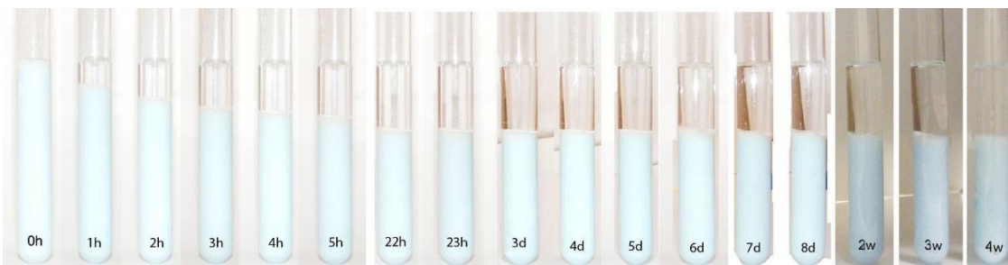
Figure 55 - Evolution of the emulsion using 8g of Pluronic P123 from 0 hours to 8 days
